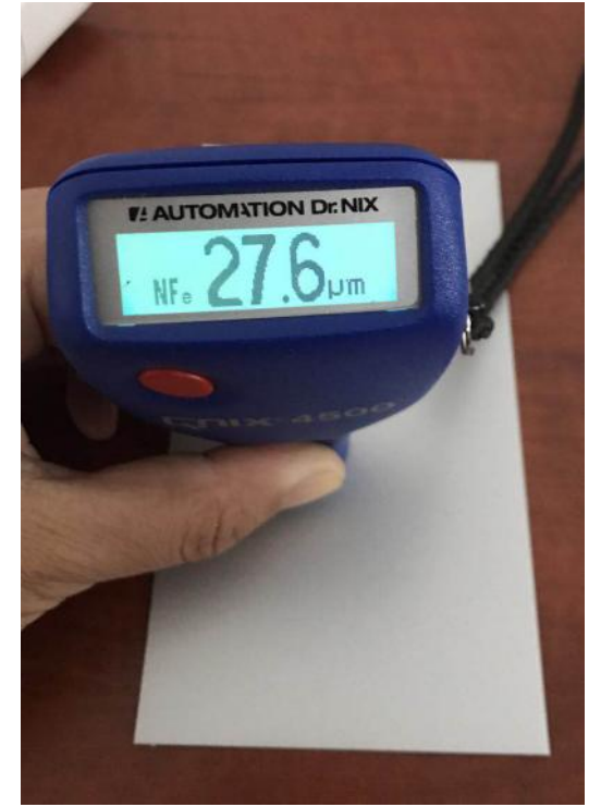
Coating Thickness Checking
